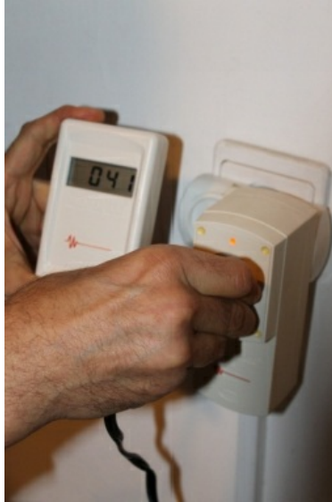
Image 5.2 Measuring again after installing a Micro-Surge Filter
