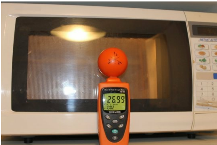
Image 6.1 - RF Radiation of an operating Microwave Oven
