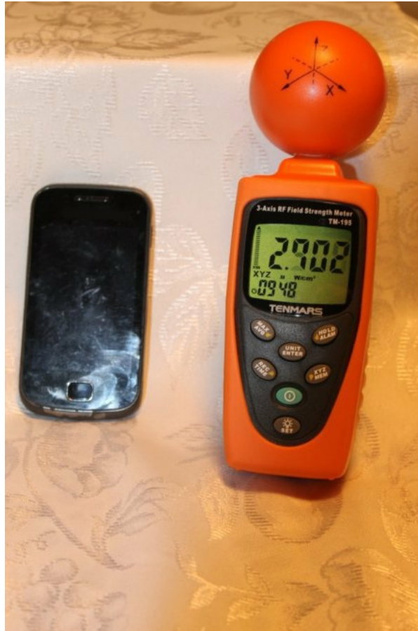
Image 7.2 - Cell Phone RF radiation (measured during initial connection phase)
