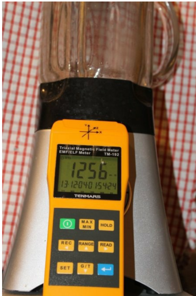
Image 4.2 - Using an LF meter to measure a blender's ELF electromagnetic radiation
